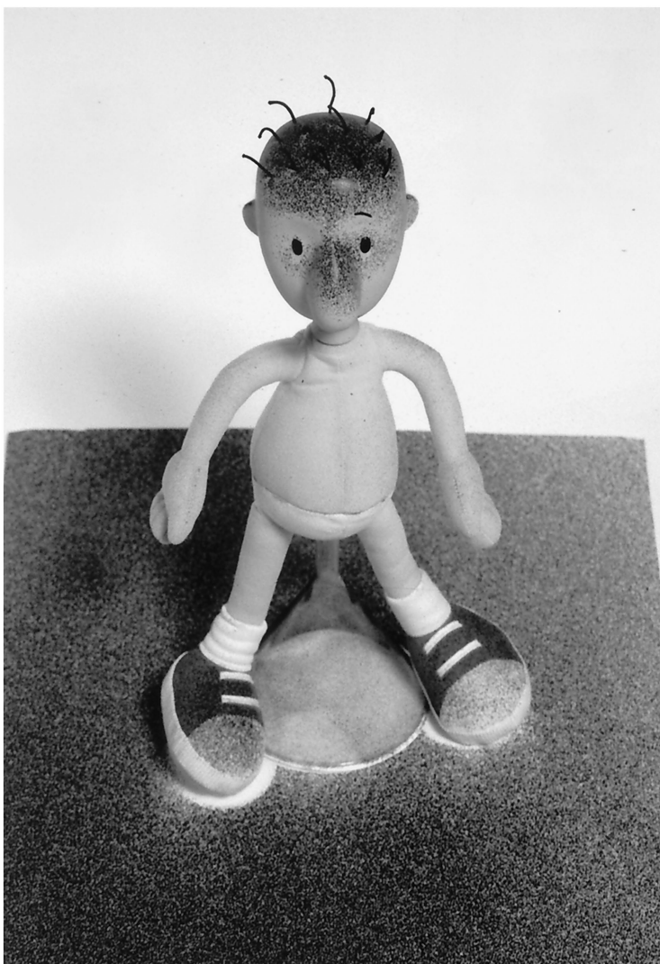
Figure 1. Deposition and distribution of spray droplets on a flat ACC and a 24" mannequin sprayed with 55 bursts of black airbrush paint at 85^\circ below the horizontal plane using a Campbell Hausfeld spray gun positioned above and in front of the mannequin.
